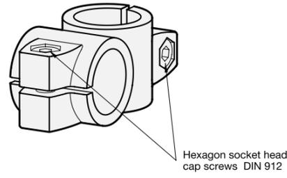
Hexagon socket head cap screws DIN 912
